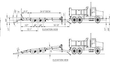
**MODEL: 25ART** 25 TON, AIR RAMP, AIR TILT, TAG NOTE: ALL DIMENSIONS ARE LOADED & NOMINAL
