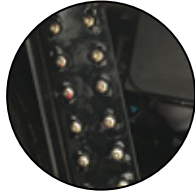
Central grease system.
