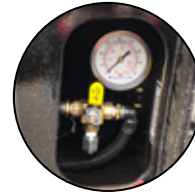
Adjustable ride height, load gauge and air suspension dump valve.
