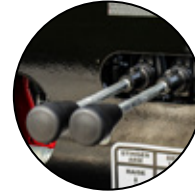
Hydraulic neck controls are easily accessible for raising and lowering trailer deck.
