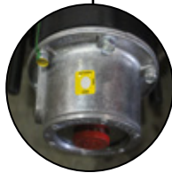
Hub alert heat detection system on the axles.
