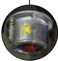
Hub Alert heat detection system on the axles.
