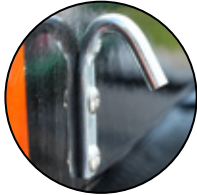
Lift Rings located on deck make it easy to stack trailers when necessary.
