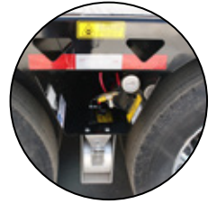
Adjustable ride height, load gauge and suspension dump valve.
