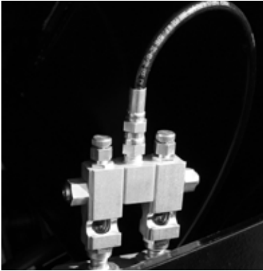
Figure 21 Oil Metering Valve
