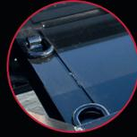
Bucket Trough with 2 Sets D Rings, in Deck Chain Box Covers
