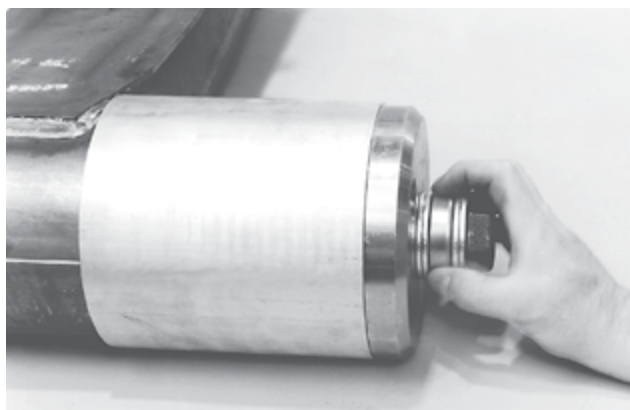
Figure 24: Ensure thrust bearing is free to turn
