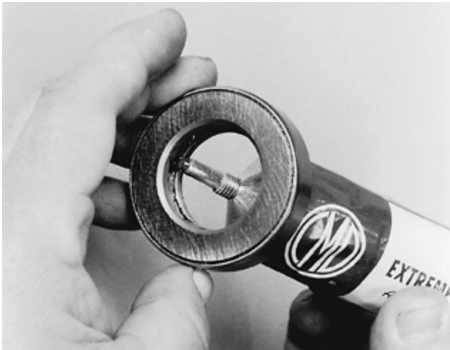
Figure 14: Applying lube to the thrust bearing
