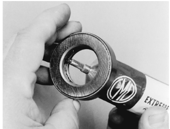
Figure 31: Applying lube to thrust bearing
