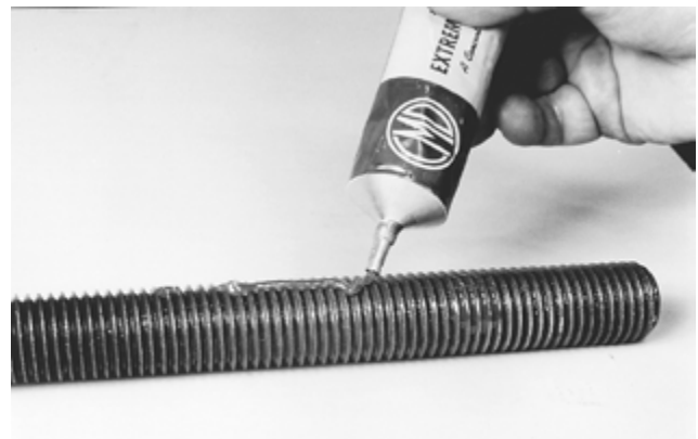
Figure 13: Applying lube to the hex head bolt
