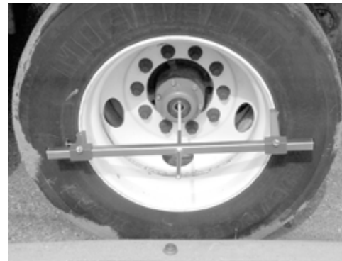
Figure 19: Installed wheel-end extender
