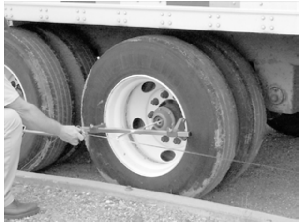
Figure 23: Measuring the "A" and "B" distances
