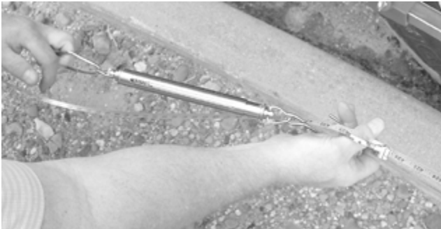
Figure 21: Using tape tension device (fish scale)
