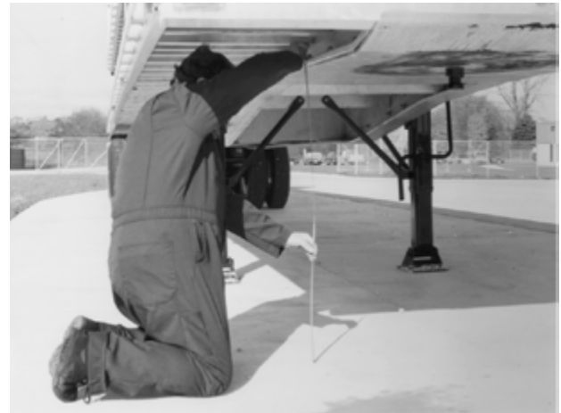
Figure 15: Measuring actual kingpin height
