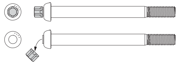
Figure 36: Shear style pivot bolt (Shown before and after shearing)
